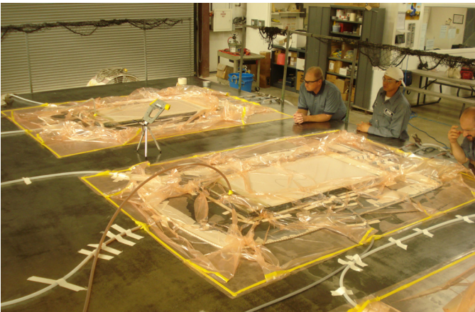
Vacuum Assisted Resin Infusion process
