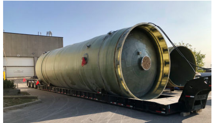
CPVC-lined chlorine drying tower
