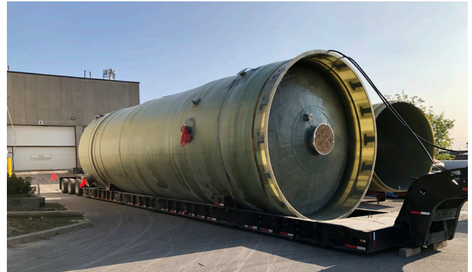
CPVC-lined chlorine drying tower
