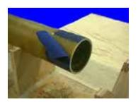
If the PEEL-A-BOND has been removed prematurely (either in transit or on the jobsite), lightly sand contaminated surface to remove any grease, oil, or other contaminant.
