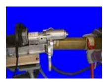
THE END OF THE TAPERED PIPE SHOULD FEATHER OUT TO 1/32" THICK FOR TAPERED ADHESIVE JOINTS, If not, adjustment of the gap between the roller (Item 20) and the grinding stone (Item 14) can be made by slackening the four (4) 3/8" diameter bolts (Item 24), readjusting for correct gap, and tightening the bolts.
