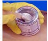
Scrape the sides and bottom of the can. Stir well, then scrape the sides and bottom again to make certain there is a thorough mixing of catalyst and adhesive or hardener and adhesive. The colder the material, the more mixing you must do.
