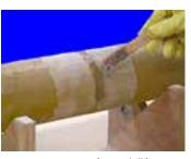
more than 1/8" by trimming the edge. At 21°C. (70°F.), the liner paste will cure in 10 to 20 minutes. In cold weather, a heat lamp should be used to achieve a proper cure.
