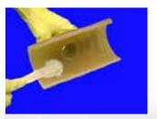
drilled hole in the pipe to aid in the corrosion protection of the pipe structure.
