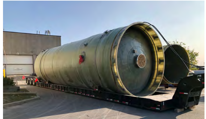
CPVC-lined chlorine drying tower
