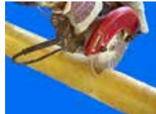
b) Field preparation is usually done using a high-speed 4 1/2" or 7" grinder, 24-36 grit (all sizes).
