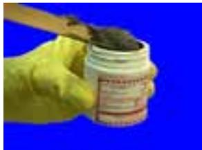
**NOTE:** The smaller kits can be mixed by hand fairly easy, but the larger kits will require a drill motor and a mixing blade to help mix the two (2) components more thoroughly.
