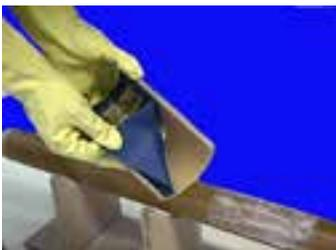
d) Mix RPS Adhesive (Refer to RPS Pipe and Fittings Installation Manual, Page 21, on general use of P1500, H1500, or E1500 adhesive).
