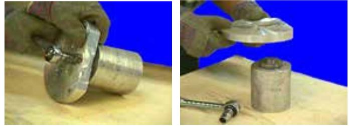
the mandrel to check the fit and ensure the pipe is level. Do not make contact with the grinding stone. Refer to "Tapering 8" - 12" Diameter Pipe", Pages 25.
