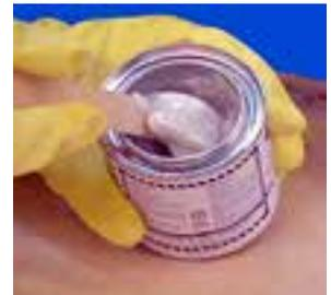
Scrape the sides and bottom of the can. Stir well, then scrape the sides and bottom again to make certain there is a thorough mixing of catalyst and adhesive or hardener and adhesive. The colder the material, the more mixing you must do.
