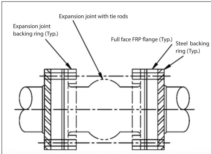
Fig 5 - Face flange connection (with backing ring) at expansion joint with tie rods
