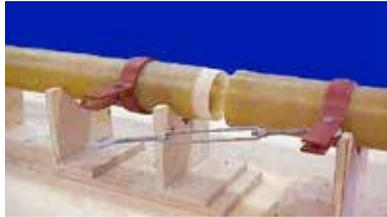
Plastic (RTR) pipe complying with B31.1 Power Piping Code or B31.3 Process Piping Code. All joints shall be made by bonders who have training in RTR piping and have satisfactorily passed the qualification tests of the appropriate code.
