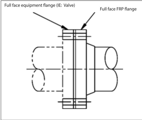
Fig 1 - Full face flange connection. Full bearing surface
