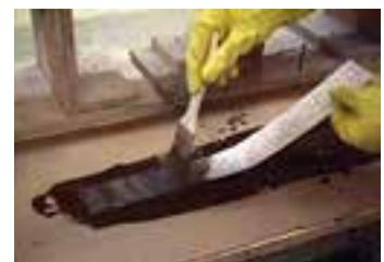
Using a paintbrush, coat a strip down the center of the cardboard sheet with a generous amount of catalyzed resin. Take the first piece (narrowest) of reinforcement and lay it binder (finished or smoothest) side up on the wet strip. Impregnate the reinforcement until all the fibers are
