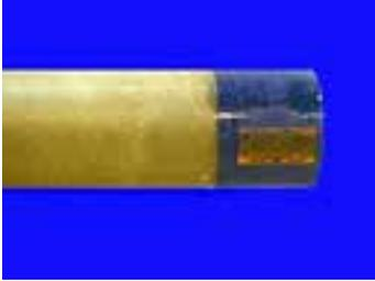
RPS pipe, fittings, or prespooled pieces may be factory prepared for field joining and protected with PEEL-A-BOND™. This eliminates the need for sanding or cleaning in the field, greatly reducing joint preparation time, and minimizing dust and noise.
